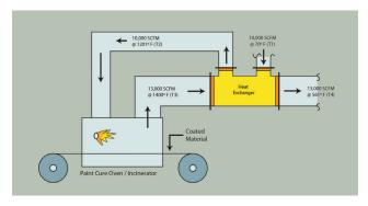
Most recovery systems can be retrofit to existing equipment, with a typical payback period of two to three years. Local utilities may have rebate programs designed to give local businesses incentives for energy efficiency improvements. Air and Liquid Systems, Inc. excels in working with all vested parties to bring added value to your heat recovery project. Our solutions bring proven technologies to the table to provide a truly low risk solution that you will reap benefits from for many years.
