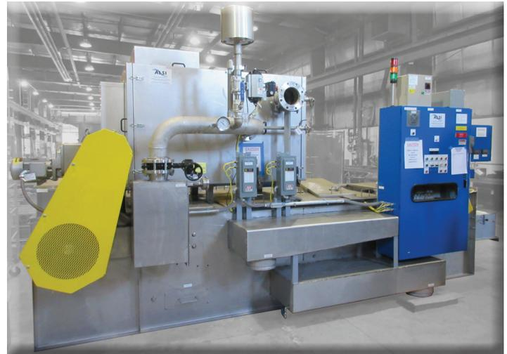
**Flat-bed Vacuum Filter with control panel**
