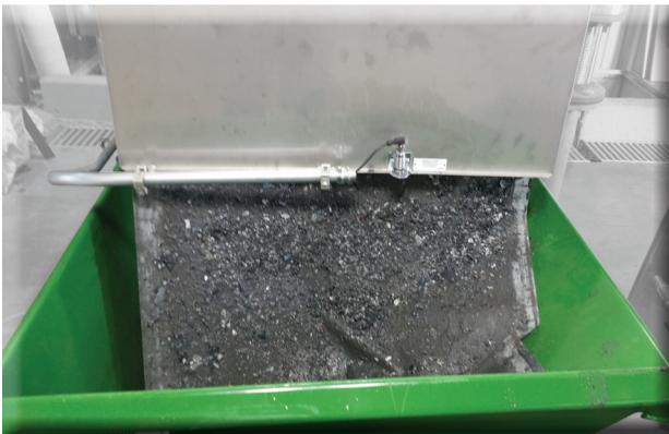
**Spent solids and media exiting Gravity Filter into receptacle**
