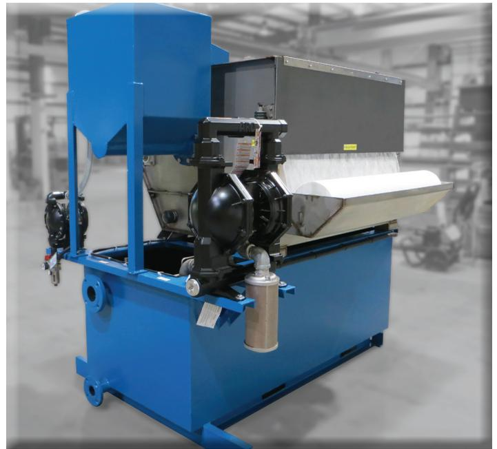
**Gravity Filter with stand and a diaphragm pump**
