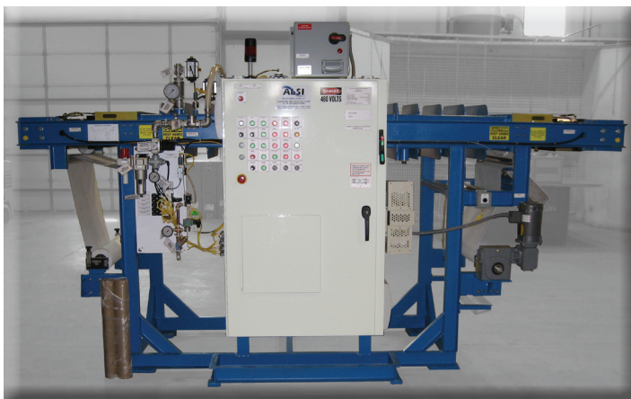
Pressure Filter with locally mounted controls
