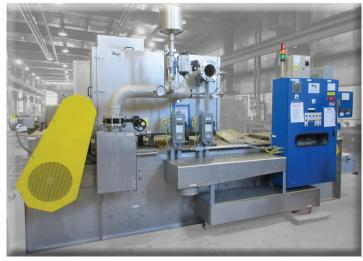
Flat-bed Vacuum Filter with control panel
