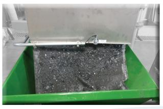
Spent solids and media exiting Gravity Filter into receptacle
