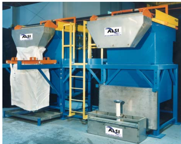
ALSI/Palin Consolidators with Dewatering Bag, Access Platform, & Autoweir (right foreground)
